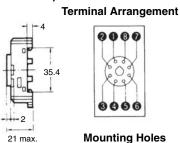
**Mounting Holes** Two, M4 or two 4.5-dia. holes 33±0.2
